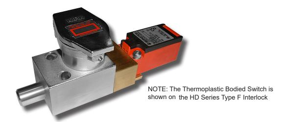
Thermoplastic bodied electrical contacts offer the best protection against water ingress. Available in 2 N/O 1 N/C or 4 N/O 2 N/C contacts. The Thermoplastic Bodies auxiliary switch can be mounted on both the SD and HD Series of the following interlocks: Type F, Type B, Type T, Type FN, Type D, Type DM.
